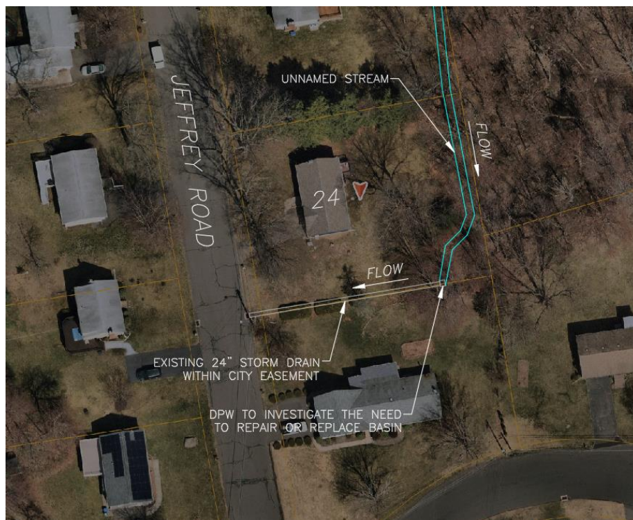
Figure 26: Proposed Drainage Improvements
