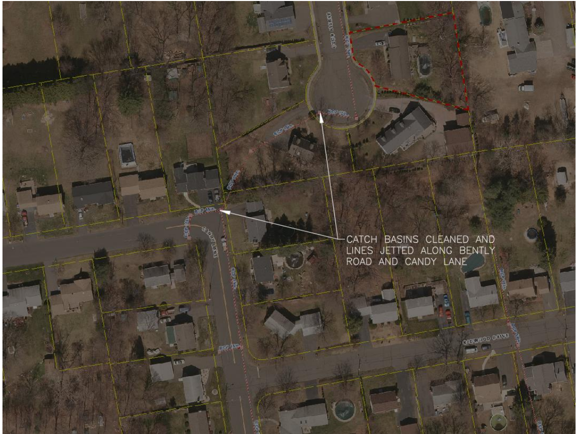
Figure 30: Maintenance of Bently Road Drainage System
