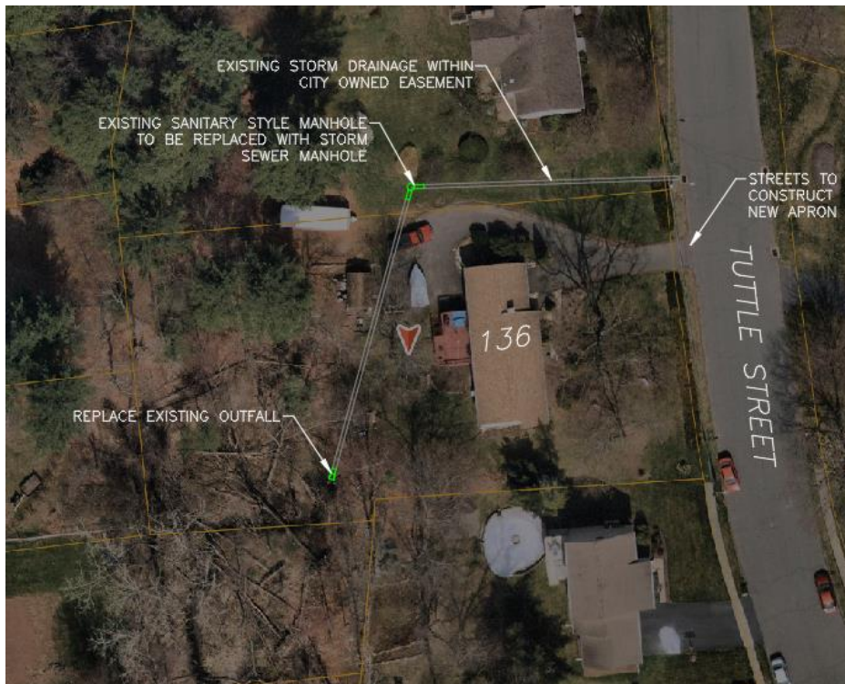
Figure 9: Proposed Drainage Improvements
