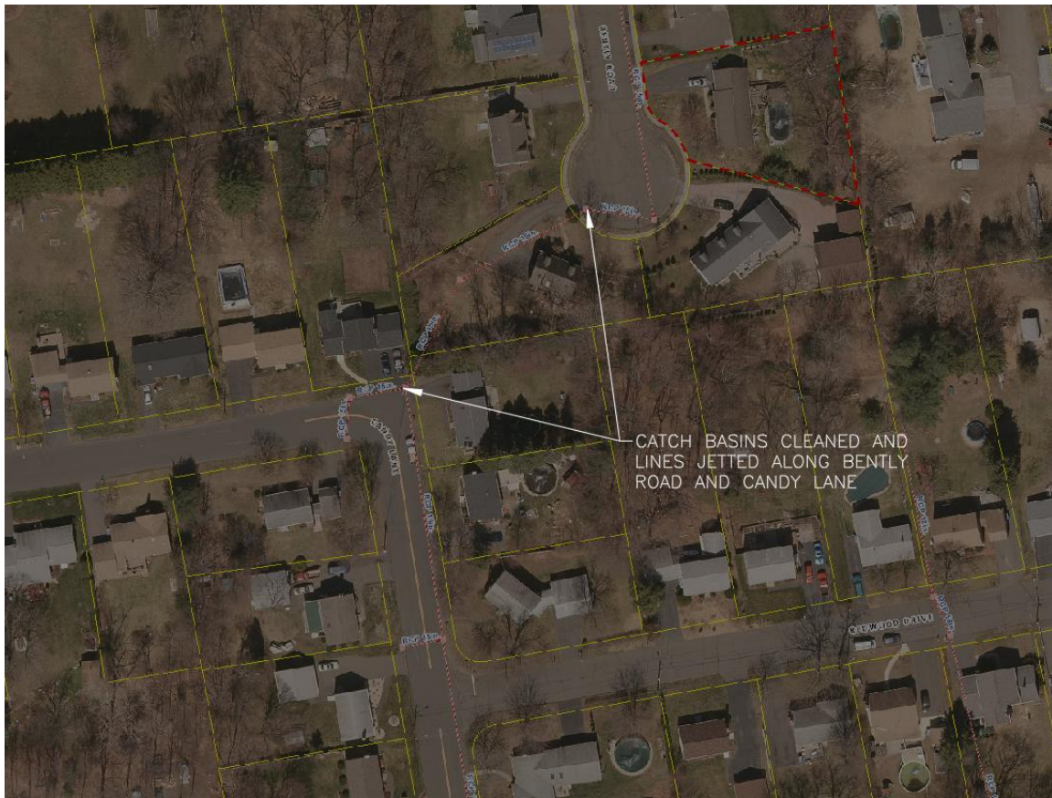
Figure 38: Maintenance of Bently Road Drainage System
