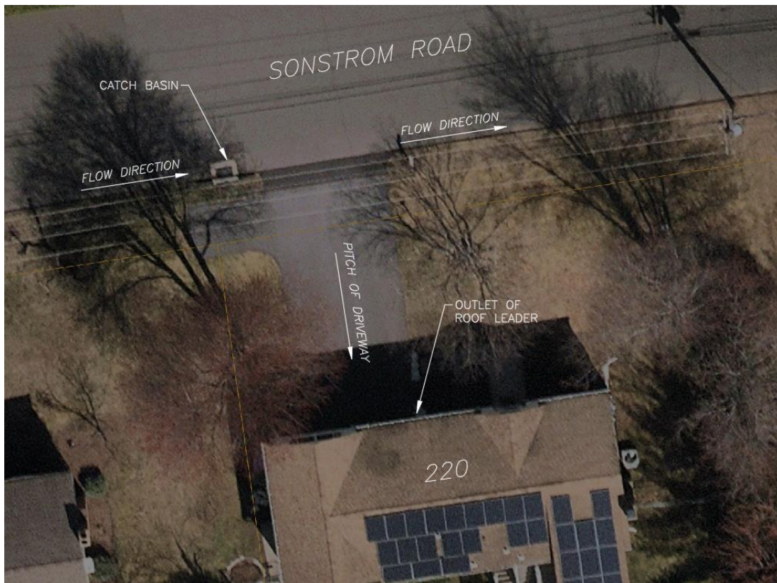
Figure 30: Site Conditions at 220 Sonstrom Road
