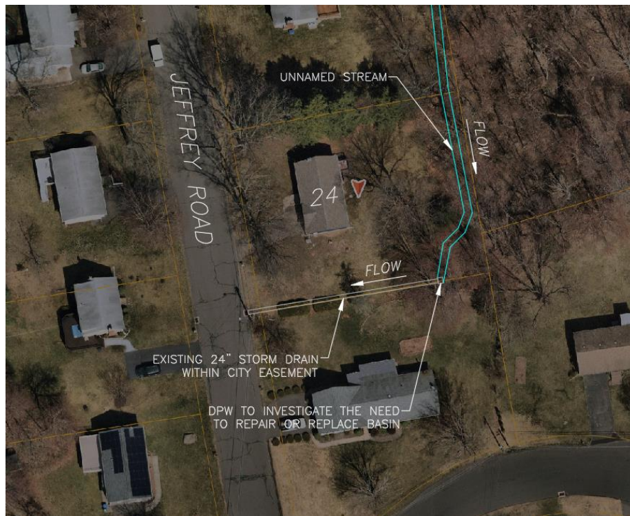
Figure 33: Proposed Drainage Improvements
