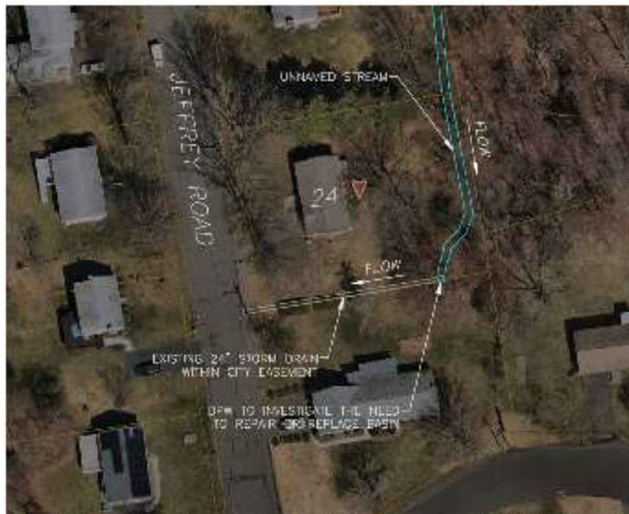
Figure 32: Proposed Drainage Improvements
