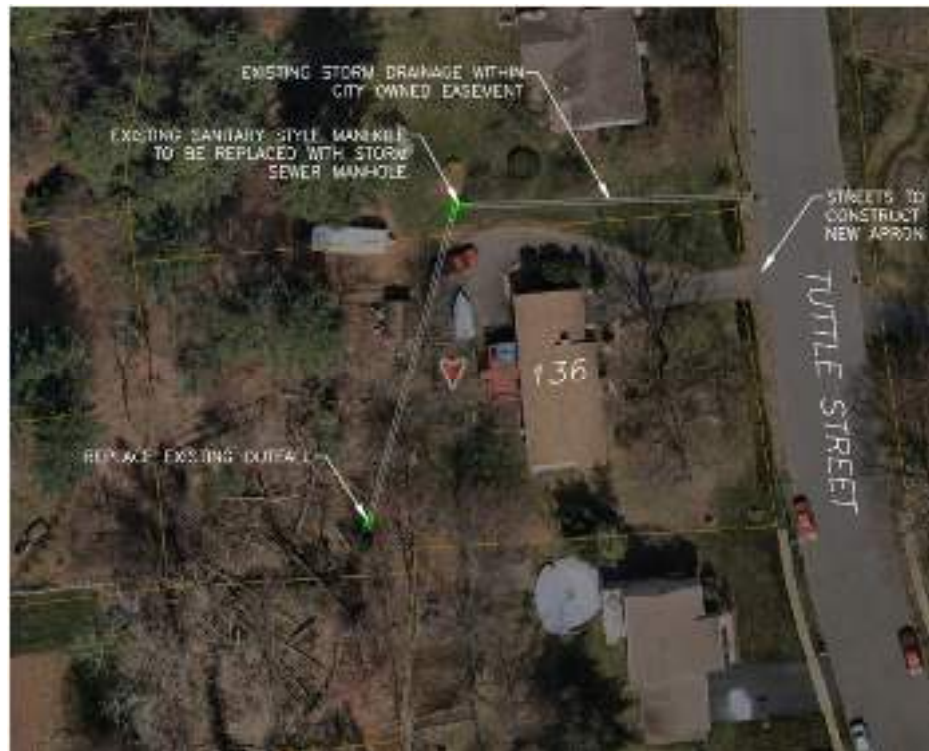
Figure 9: Proposed Drainage Improvements
