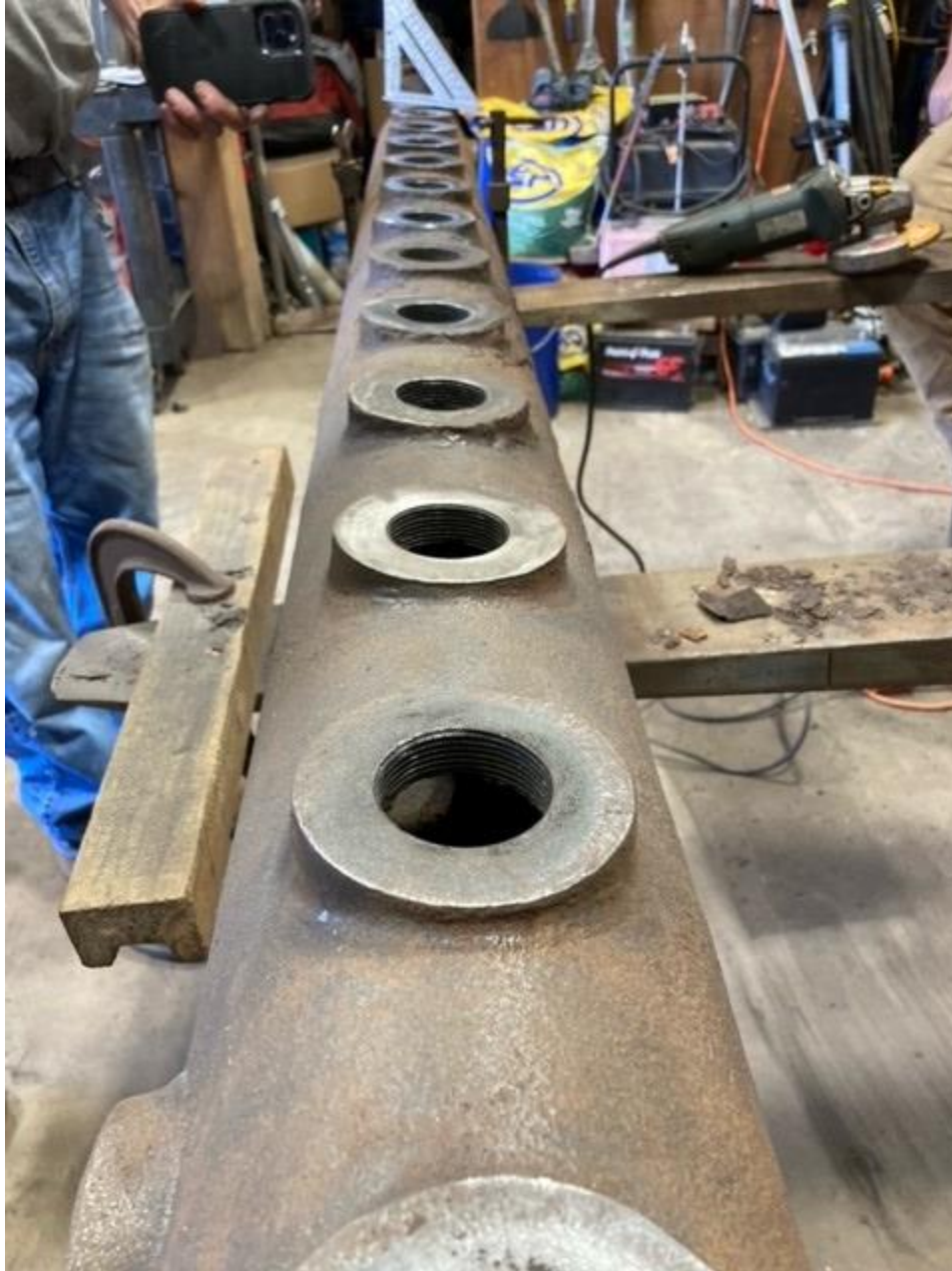
Mud drum after re-conditioning at Oakland LLC
