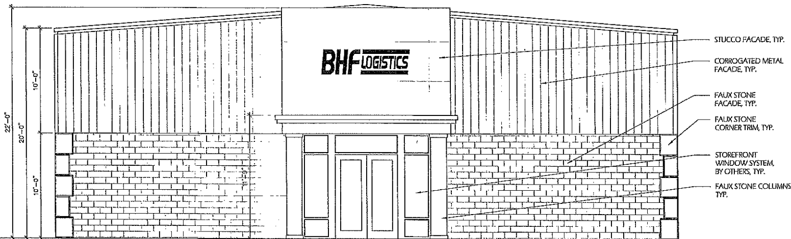
E1 FRONT EXTERIOR ELEVATION 1/4" = 1'-0"
