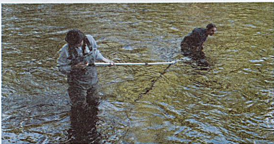
Ciara and Paige measure flow in the River
